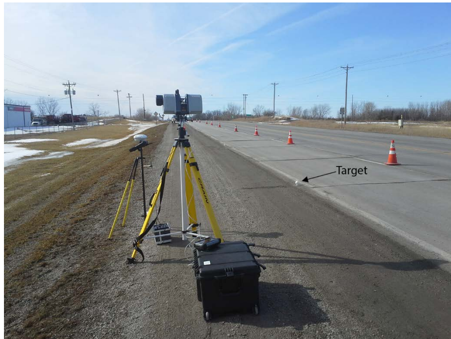
Figure 5. Laser scanner setup at “rough” pavement section showing scanner, GPS equipment and targets.
